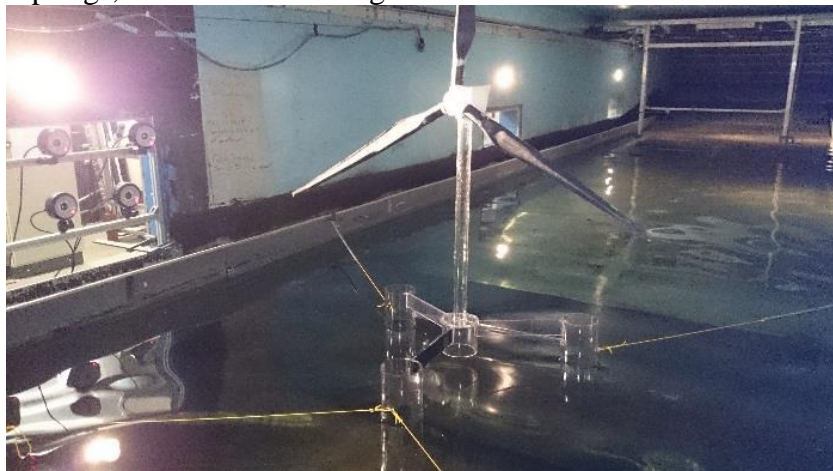
Figure 9 Floating wind turbine in the wave and wind flume with the trajectometry cameras
